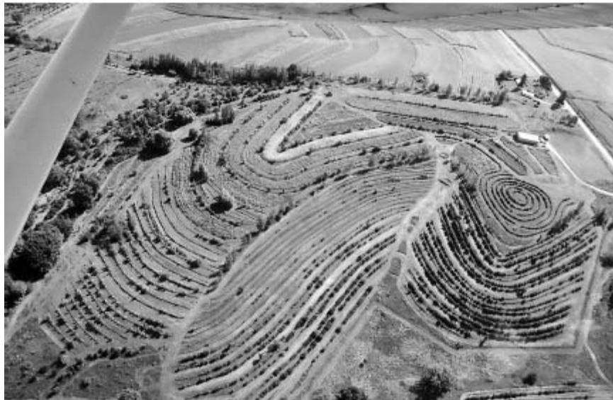
Keyline swales, berms and pocket ponds capture and spread out all rainwater while allowing access for vehicles, water lines, and livestock fencing while creating a beautiful, functional farming landscape.
